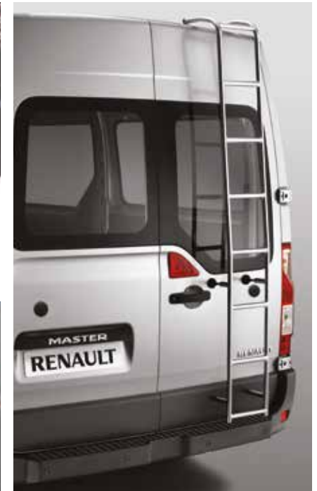
Walkway and Ladder
